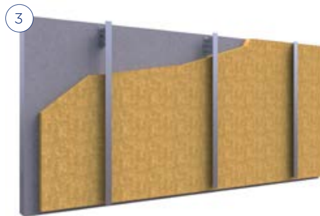
Fastening the "L" shaped vertical profiles
